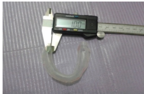
Figure 3: One mm thickness of vacuumed polyethylene sheet.
